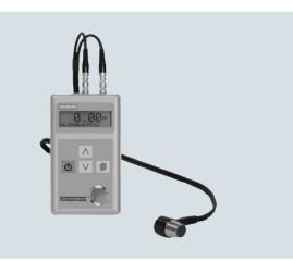
The thickness gauge is used to measure the wall thickness of the pipe that a clamp-on ultrasonic flowmeter is installed on. The wall thickness value is a vital factor in the flow computation model and a prerequisite for precise clamp-on ultrasonic flow measurement. When measuring any pipe wall thickness the thickness gauge can also be used as a stand-alone tool used to measure the wall thickness of any metallic or non-metallic pipe materials capable of acting as an ultrasonic wave conductor.
